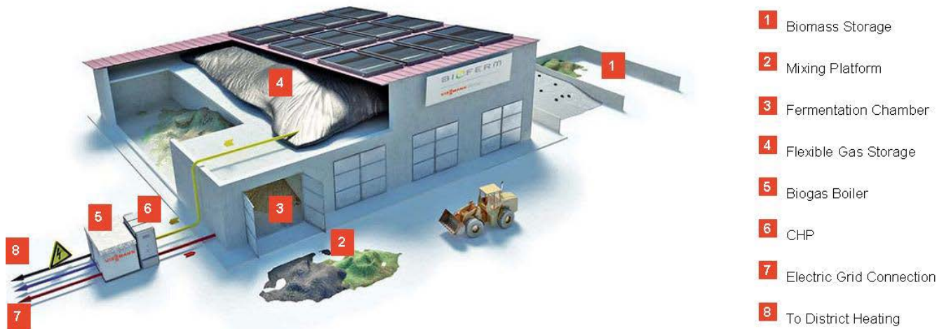
Figure 3-1: Example of Garage Style Dry Anaerobic Digestion
