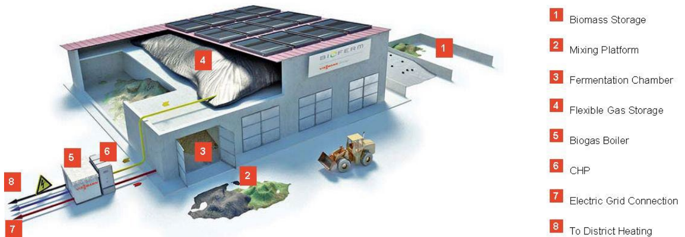
Figure 4.4-5: Example of Garage Style Dry Anaerobic Digestion
